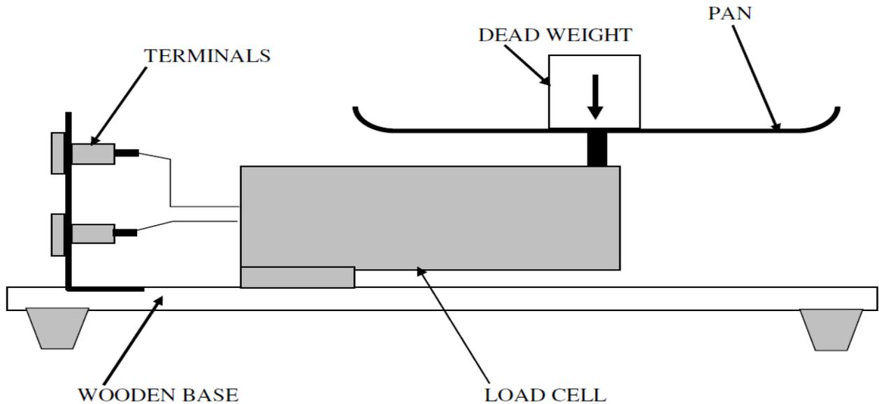
**BEAM TYPE LOAD CELL MOUNTED ON A WOODEN BASE****OPERATING PROCEDURE:**
