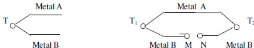
The electric potential is usually measured by introducing a special junction in an electric circuit. The voltage across terminals M-N can be represented approximately by an empirical equation having the form.
